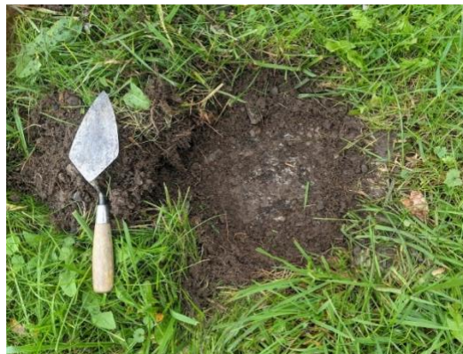
Photo 8: Disturbed Test Pit, buried asphalt
