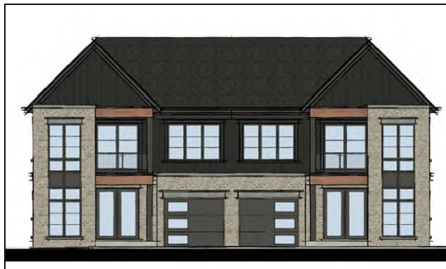
Figure 10 - Preliminary 2-storey Townhouse Front Elevation
