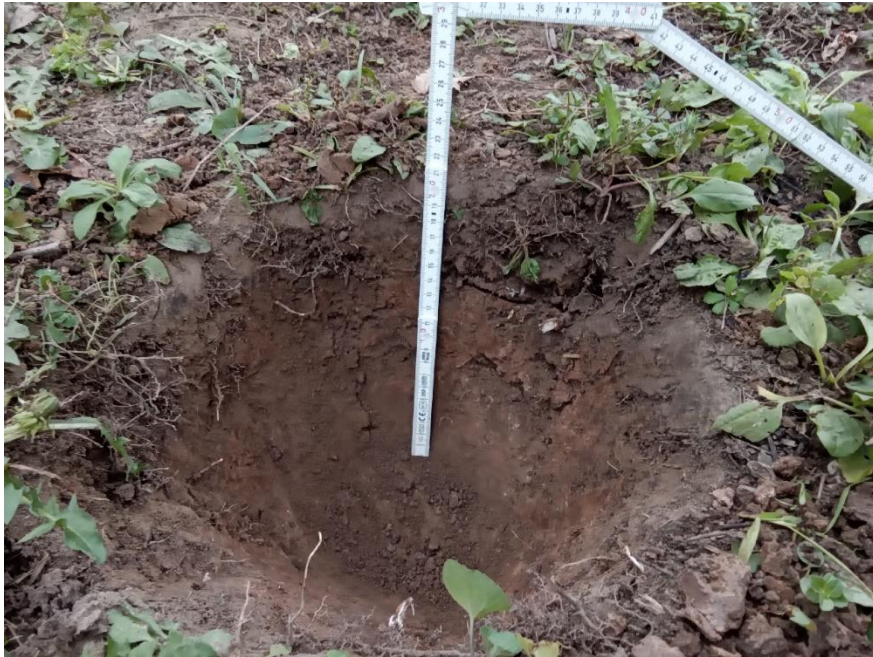
Image 11: Test pit soil profile in the southwest of the subject property, adjacent to the driveway.
