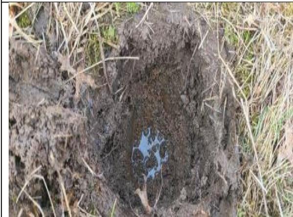
**IMAGE 9 LOW-LYING WET AREA TEST PIT IN PROGRESS**
