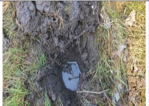
**IMAGE 4 LOW-LYING WET AREA TEST PIT IN PROGRESS**
