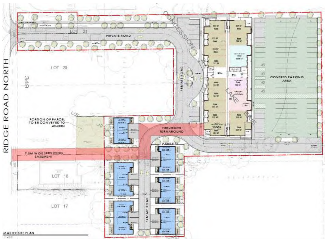
FIGURE 14: PORTION OF THE SITE PLAN DEPICTING THE LAYOUT OF THE PROPOSED REDEVELOPMENT
