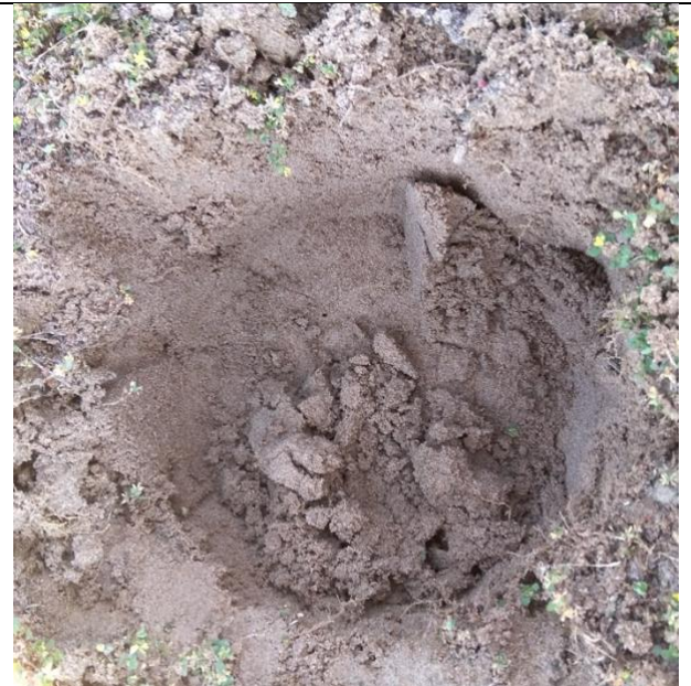
IMAGE 8 TEST PIT IN PROGRESS: SAND FILL, DISTURBED
