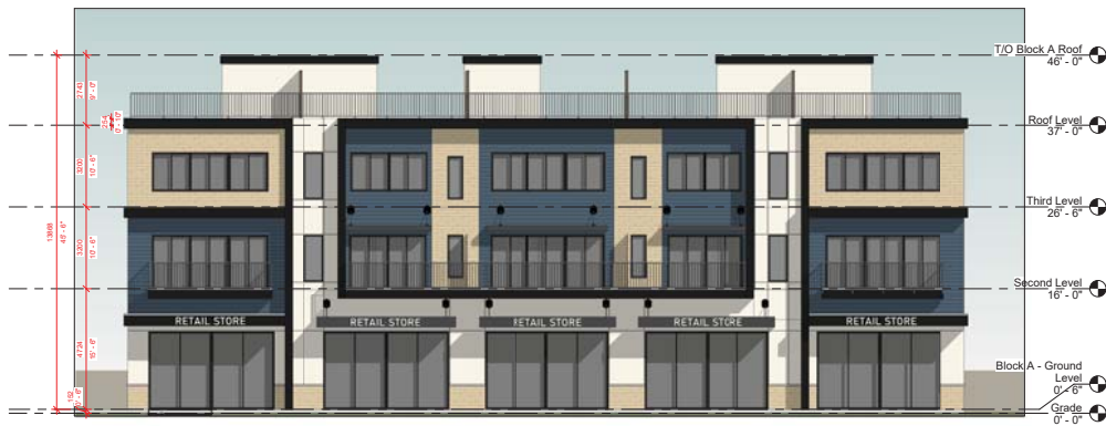
1 Block A - North Elevation (Front) 1 : 100
