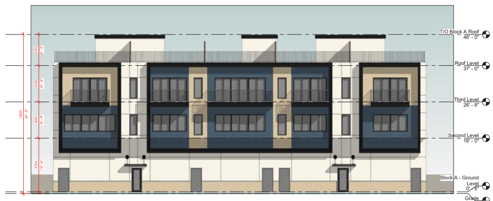
2 Block A - South Elevation (Rear) 1 : 100
