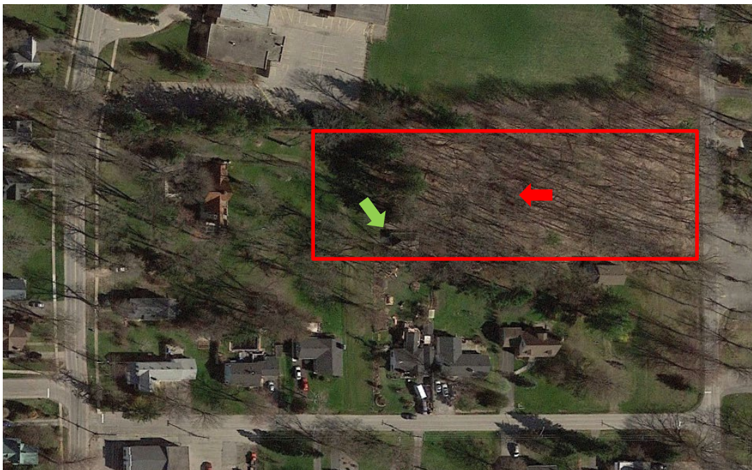
Figure 13: Portion of 2017 aerial image, red outline denotes approximate limits of Subject Property and red arrow indicates the location of the cement lined depression. Green arrow indicates a structure that is no longer present
