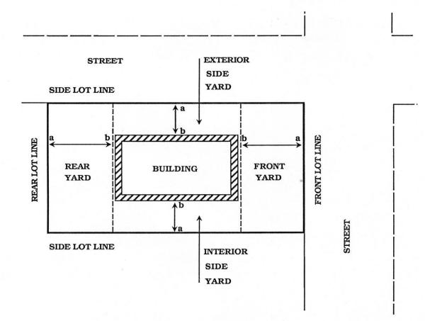
DISTANCE ab REPRESENTS THE DEPTH OF THE REQUIRED YARD MEASURED AS LEAST HORIZONTAL DIMENSION BETWEEN LOT LINE AND NEAREST PART OF MAIN BUILDING. DISTANCE ab MUST BE THE MINIMUM DISTANCE SPECIFIED IN BY-LAW.
