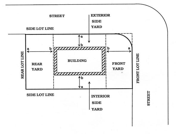
DISTANCE ab REPRESENTS THE DEPTH OF THE REQUIRED YARD MEASURED AS LEAST HORIZONTAL DIMENSION BETWEEN LOT LINE AND NEAREST PART OF MAIN BUILDING. DISTANCE ab MUST BE THE MINIMUM DISTANCE SPECIFIED IN BY-LAW. 6.52
